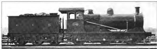
Fig. 5030. Six-Coupled Goods Locomotive. Great Eastern Railway. Cylinders-19 in. x 26 in.; Total Heating Surface 1,706.58 sq. ft.; Diameter of Drivers 59 in.; Weight on Drivers 102,080 lbs.; Total Weight 102,080 lbs.
